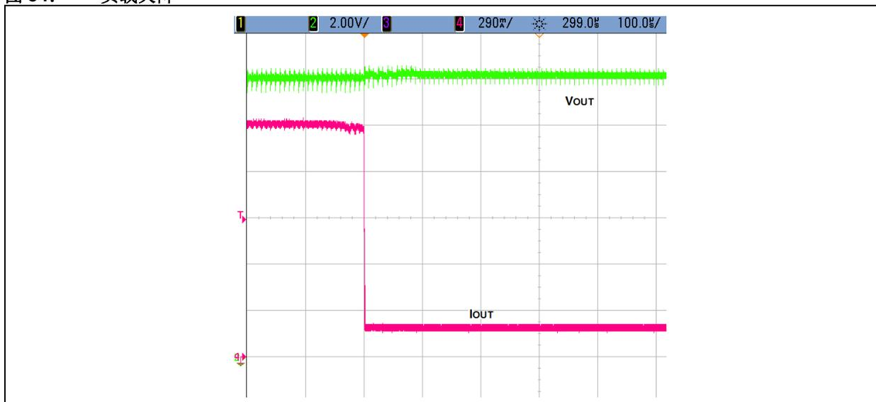
图 85: 输入电压开关期间的  $V_{out}$
