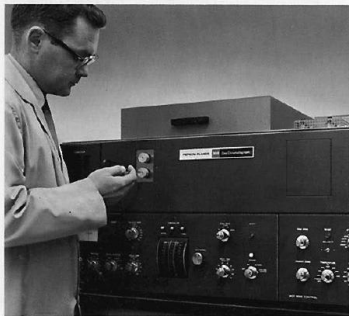
Chianti, vintage 1957, is introduced into the gas chromatograph. Comparison of differences in trace components on the chromatograms may be related to differences in relative quality of individual vintages.
