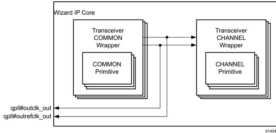
Figure 3-8: Transceiver Common Located in the Core
