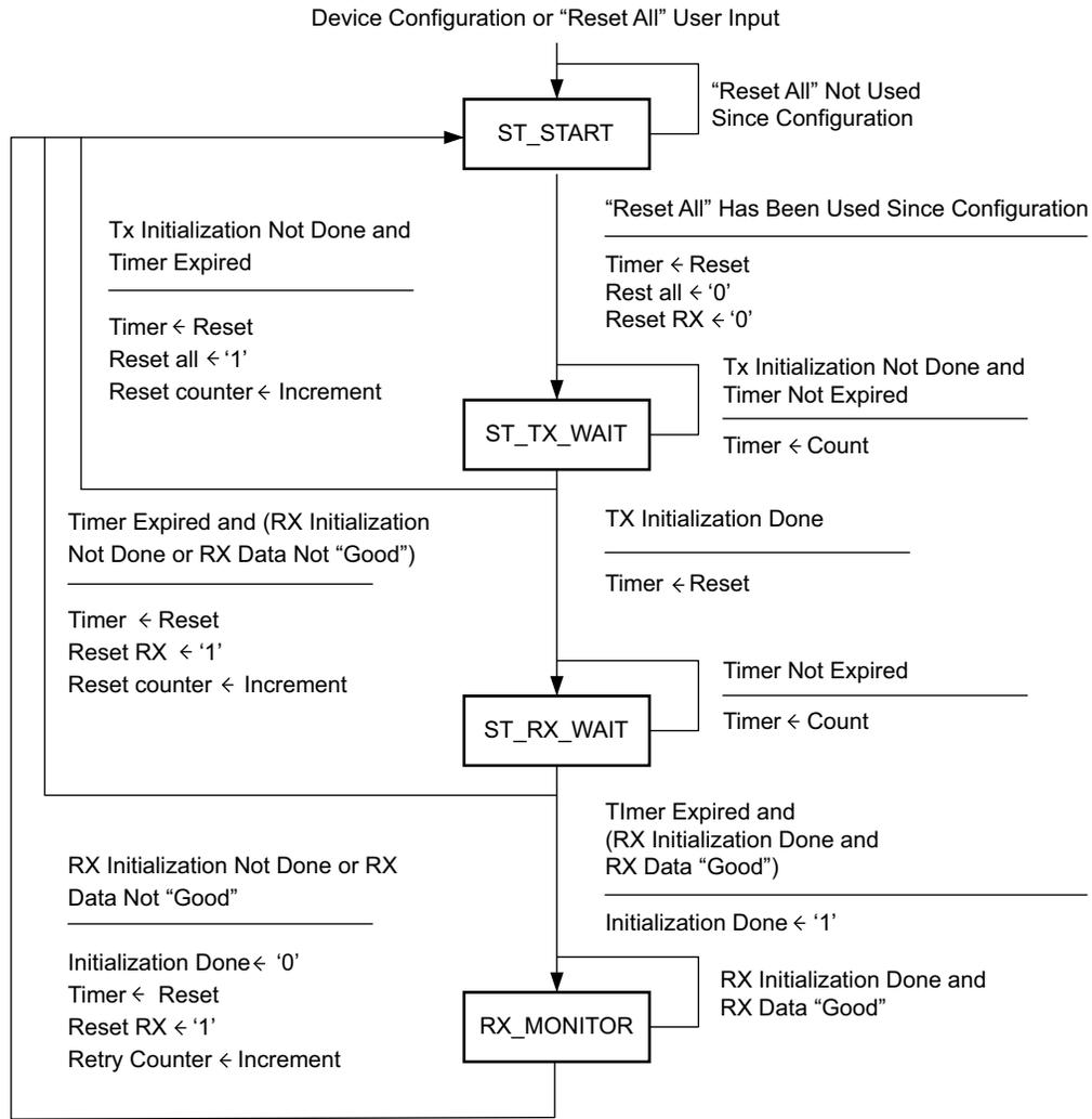
Figure 5-3: Example Initialization Module Finite State Machine
