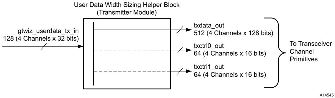
Figure 3-6: User Data Width Sizing Helper Block (Transmitter Module) Example Configuration
