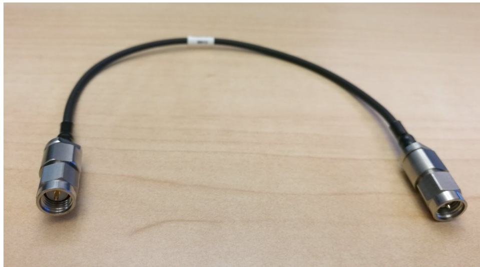
Figure 34: SMA to SMA Cable: Carlisle TM40-0159-00 6"
