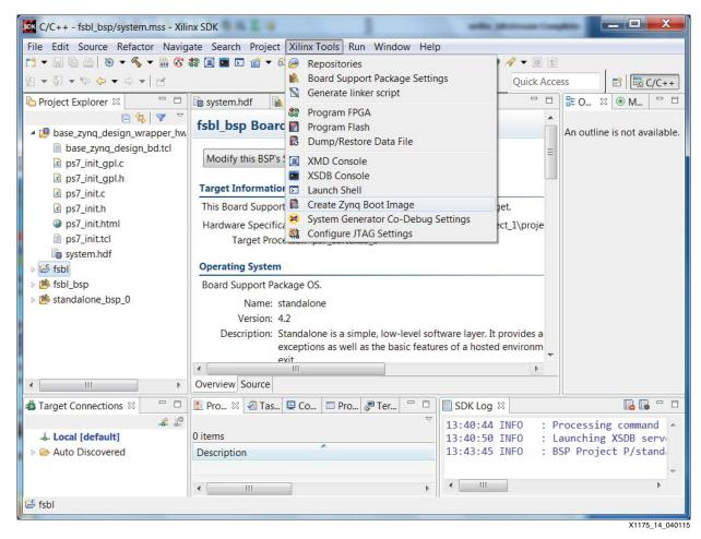
Figure 16: Invoking Bootgen
