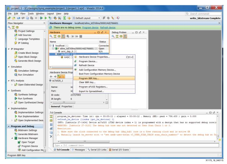
Figure 20: Using Vivado Hardware Manager to Program the BBRAM Key
