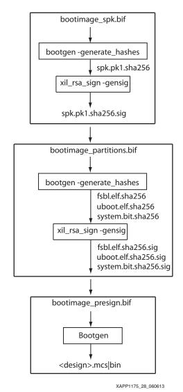
*Figure 33:* **Bootgen Release Mode Flow**
