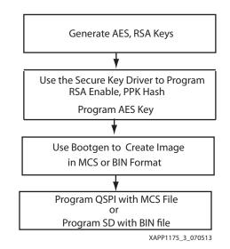
Figure 3: Steps in Developing a Secure System
