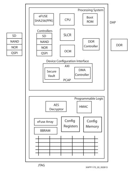
Figure 2: Zynq-7000 SoC Hardware Components Used in Boot
