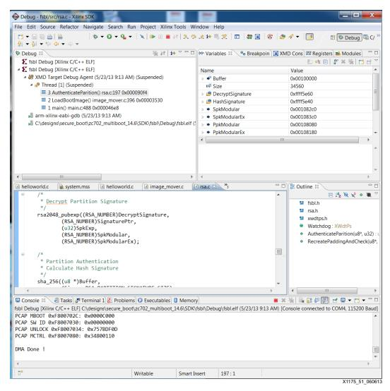
Figure 45: RSA Verification of Partition
