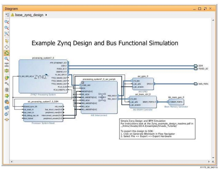
Figure 11: Zynq Example Board Design Schematic
