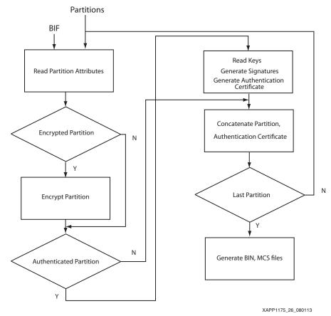
Figure 24: Bootgen Flow Diagram
