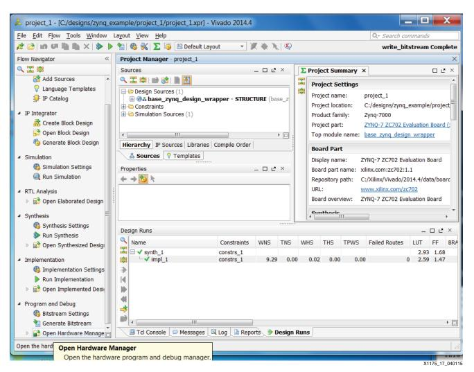
Figure 19: Opening the Hardware Manager in Vivado
