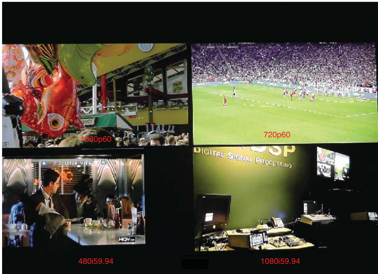
Figure 6: Four Video Standards Passed Through and Displayed
