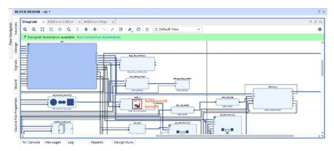
The following image displays the implemented design view of the hello\_world kernel hooked to a flat shell. Note that there are no partitions in the implemented design.
