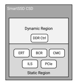
Figure 2: Target Platform Shell Dynamic and Static Regions
