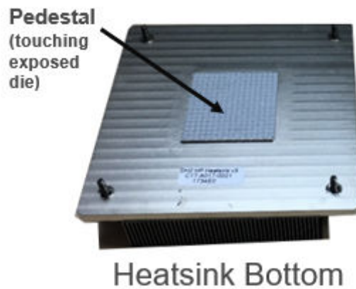
Figure 13: Pedestal Extruding from Heatsink Base
