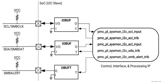
Figure 19: Connecting I2C/PMBUS to SelectIO Package Pins
