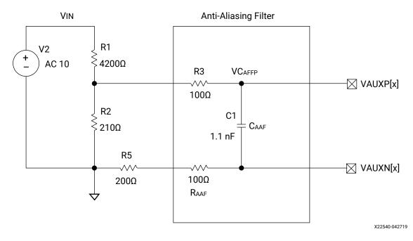
*Figure 13:* **Anti-Alias Filter and Voltage Attenuation**
