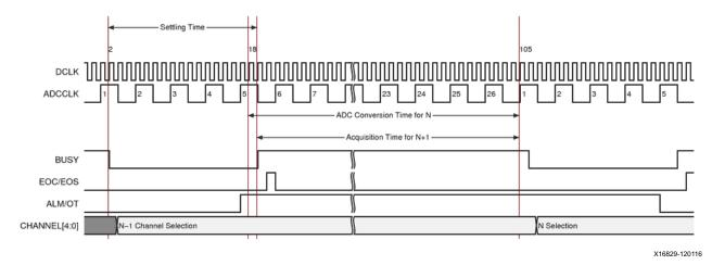
Figure 2-5: Continuous Sampling Mode
