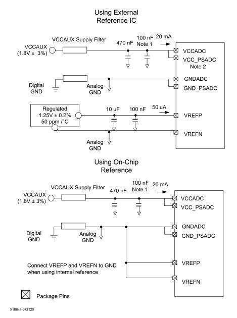
Figure 5-1: ADC Power and Ground Connections
