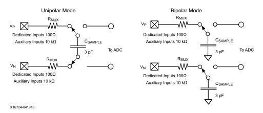
Figure 2-7: Equivalent Analog Input Circuits (shown as SYSMONE1)
