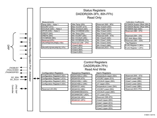
Figure 3-1: SYSMONE1 Register Interface
