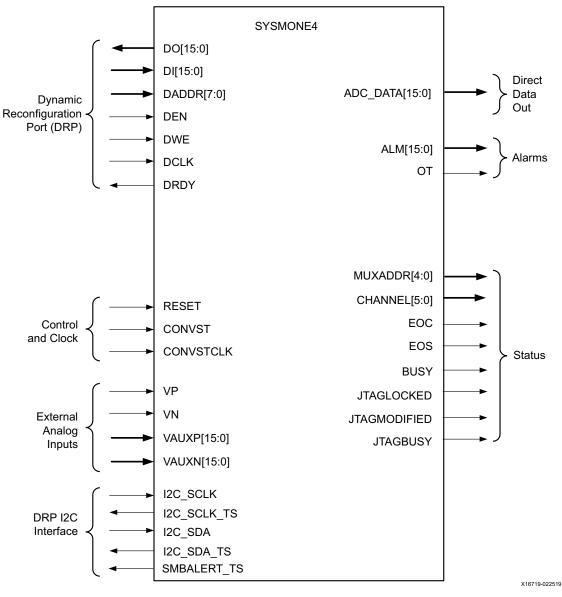
Figure 1-5: SYSMONE4 Primitive Ports
