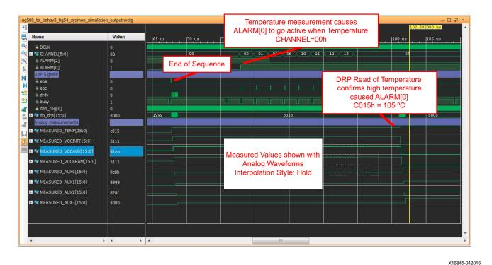
Figure 5-4: SYSMON Simulation Output
