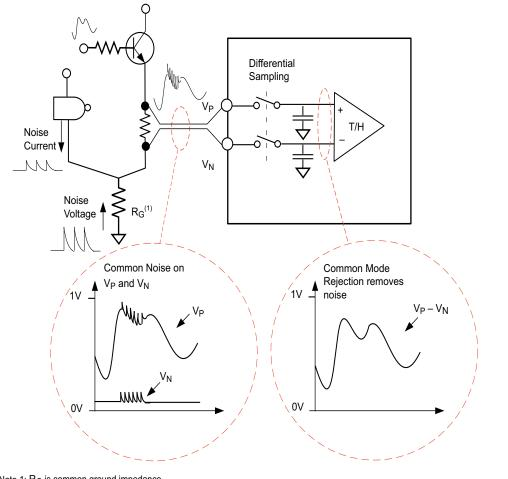
Note 1:  $R_G$  is common ground impedance.
