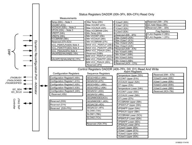
Figure 3-2: SYSMONE4 Register Interface
