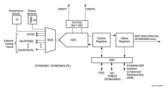
Figure 1-1: SYSMONE1, SYSMONE4 (PL) Block Diagram
