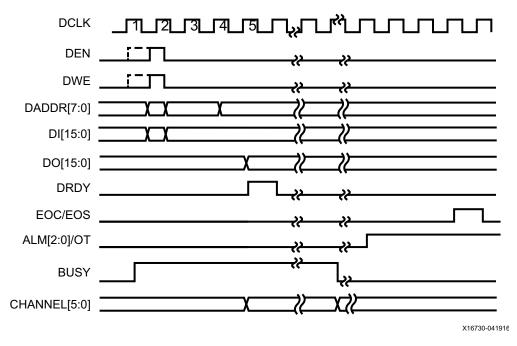
Figure 3-3: DRP Detailed Timing
