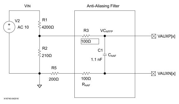
Figure 5-3: Voltage Attenuation
