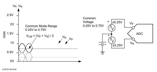
Figure 2-10: Differential Input Signal Range
