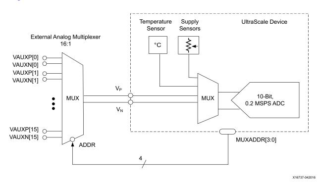
Figure 4-3: External Multiplexer Mode
