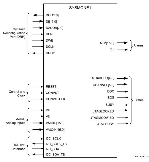
Figure 1-4: SYSMONE1 Primitive Ports
