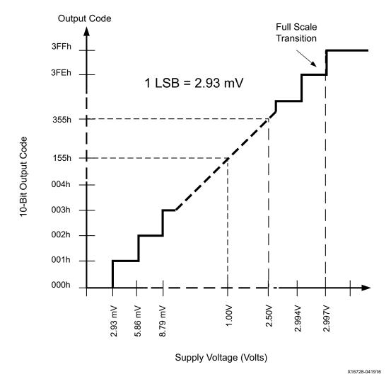
*Figure 2-11:* Ideal Power Supply Transfer Function (All Supplies Excluding HR I/O Banks (SYSMONE1), HD I/O Banks (SYSMONE4), and V<sub>CCO PSIO</sub> (Zynq UltraScale+ MPSoC PS Block))
