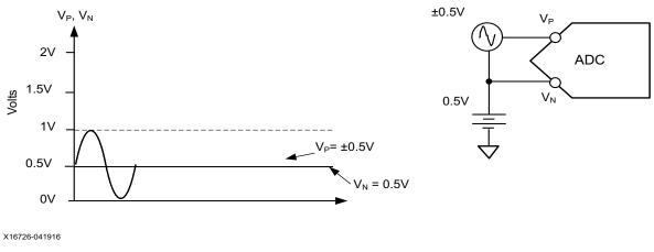
Figure 2-9: Bipolar Input Signal Range
